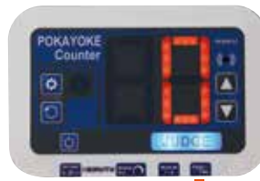
When the task count of the registered work becomes '0', the counter outputs PASS. If the counter overcounts, the counter outputs FAIL.
