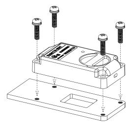
When using metal as fixing material, it is recommended to use metal with plate thickness of 2 mm or more (1mm or more for burring). For transmitter fixing screws, pan small screws with spring washer M3\*10 mm or larger are recommended.
