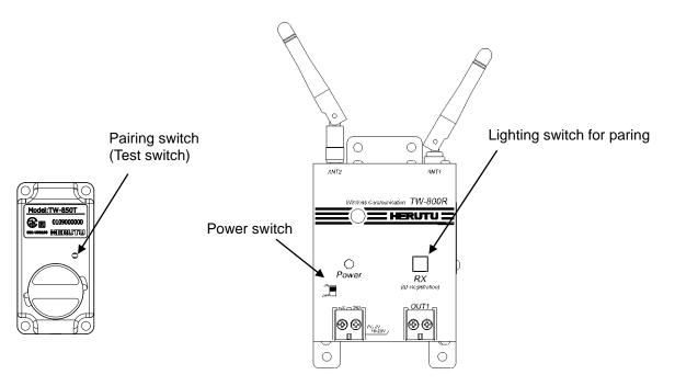
②Long press the pairing switch of the transmitter for 3 seconds or longer.
