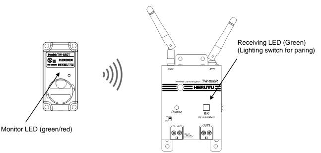
②A wireless signal is transmitted by inputting a work completion signal to the transmitter.
